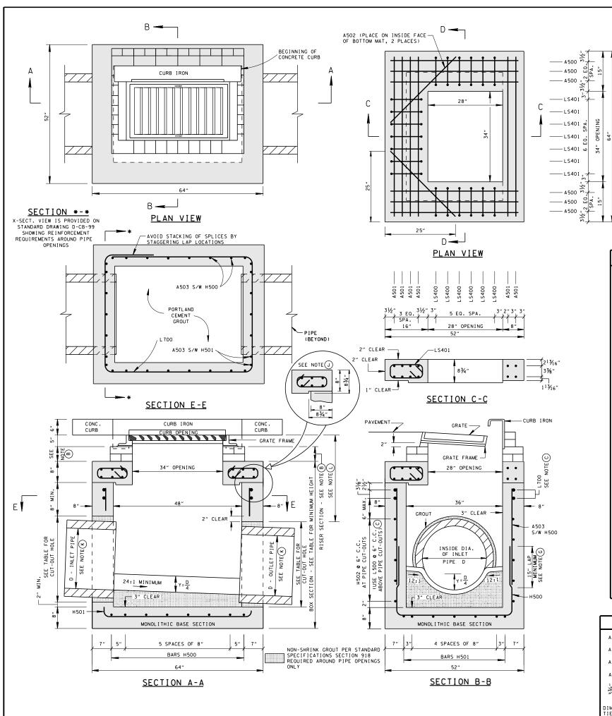
CATCH BASIN MAXIMUM DEPTH NOTE MAXIMUM DEPTH FOR THIS STRUCTURE IS 20.00'
